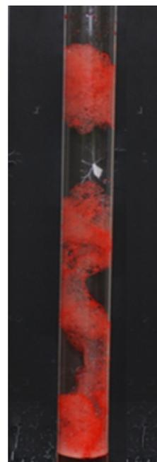
**Fig. B.1.** Non-uniformed breakdown of foam made with Cocobetaine in the presence of Isopar N. This image highlights one of the major challenges in quantifying foam height in the bulk-scale experiment. The foam in the column is no longer representative of the true foam height. Although the data obtained from this image was not included in the analysis, this phenomenon occurred multiple times and posed a difficulty in quantifying the foam height accurately.
