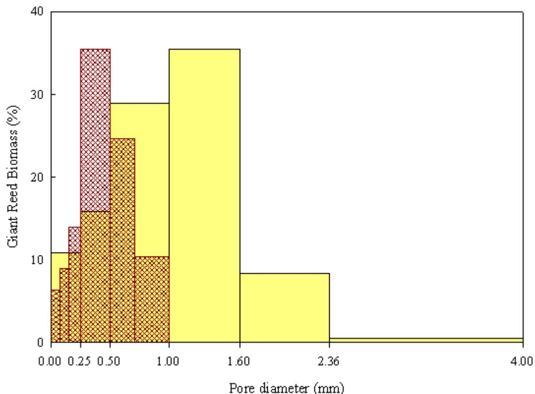
Figure 2.A. donax particle size distribution using 1mm (red/dotted) or 4 mm (yellow/filled) milling sieves.
